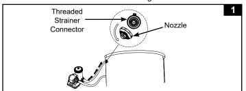
Make sure the micro-screen (6) is inside the hose adaptor (7), then screw the hose adaptor to the threaded strainer connector, from inside of the pool. See Fig. 2.
