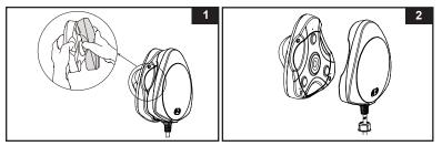
2. Place the transmitter (2) on the outside of the pool wall and the pool light (1) on the inside of the pool wall submerged in water. Ensure the transmitter magnetic poles are properly aligned with the magnetic poles on the pool light unit. See drawing (3).
