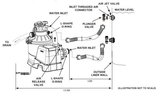
According to the International Standard, IEC 60364-7-702, on electrical installation of swimming pools and other basins equipment, the following installation distances must be respected:
