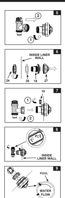
**NOTE:** Do not cover the air jet valve **(15)** with the valve cap **(34)** under normal situation or when the pump is operating. See Troubleshooting Guide section for more details.
