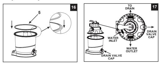
IMPORTANT: There are three hose connection ports on the 6-way valve, ensure the outlet connection (from filter to the pool) on the valve is facing towards the pool (see drawing 18).
